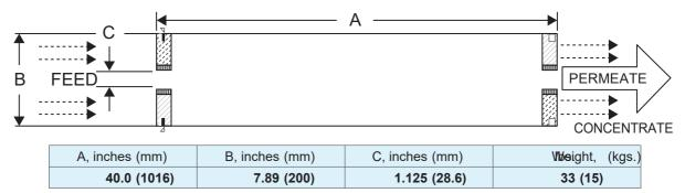
**Notice:** Permeate flow for individual elements may vary ±15 percent. Membrane active area may vary ±4%. All membrane elements are supplied with a brine seal, interconnector, and o-rings. Elements are enclosed in a sealed polyethylene bag containing less than 1.0% sodium meta-bisulfite solution, and then packaged in a cardboard box.
