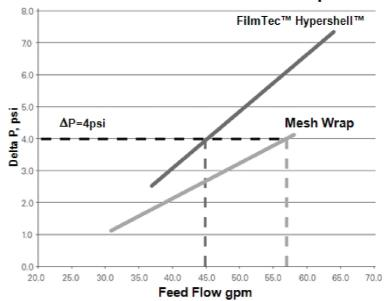
Pressure Drop versus Feed Flow for Mesh wrap and FilmTec<sup>™</sup> Hypershell<sup>™</sup> 8038 elements. FilmTec<sup>™</sup> Hypershell<sup>™</sup> has less exterior bypassing and requires approximately 30% less flow than mesh wrap for an equivalent pressure drop.
