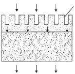
Surface structure spreads water flow and increases filtration area.
