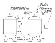
NOTE: Flexible connectors must be installed between hard piping and tank openings. These pressure vessels are treated for an internal negative pressure of 5y HG (17 Pa) vacuum below atmospheric. If negative pressure could ever exceed 5y Hg (17 Pa), an adequate vacuum breaker must also be properly installed. Failure to install flex connection properly, or improper installation of a vacuum breaker when required, may void the warranty.
